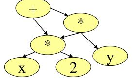
Powerful representation, encodes redundancy; but difficult to transform, not useful for showing control-flow.
